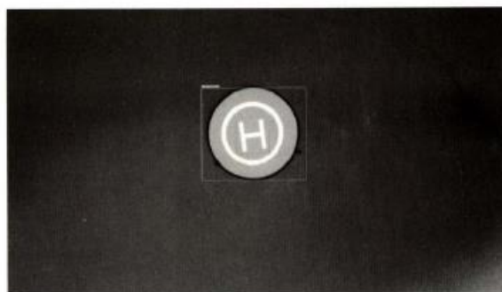
Figure 4. Tarmac recognition results from UAV view
