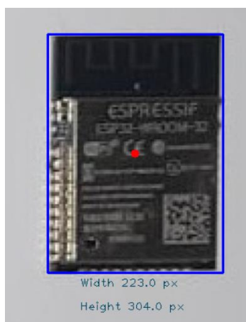
Figure 1. Microcontroller contour detection by OpenCV system
