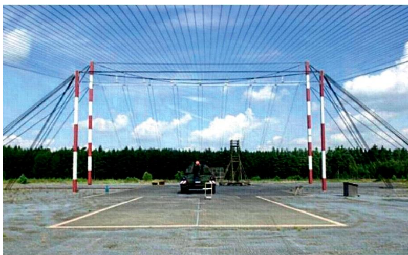
Figure 11. The antenna system of the test bench simulating HEMP
