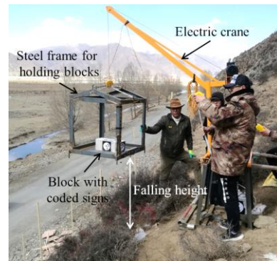
Figure 2. Automatic release apparatus for rockfall
