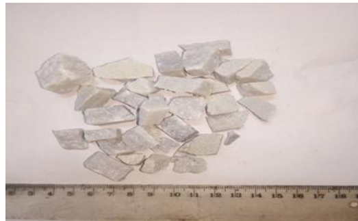
Figure 2. Coarse RMA after crushing.
