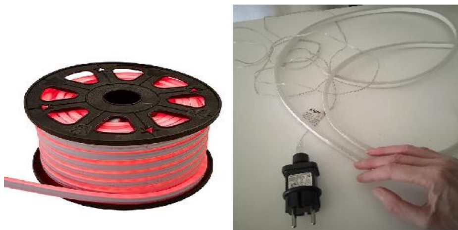
Figure 1. Left: The material for a LED-tube; (LEDs of 0.02W inside a soft elastomere). Right: A part ~2.5m and 6W, that provides enlarged temperature. At motion, it feels electric prior to desired extra heat. Possibly, additional arrangements could be done to obtain more heat from such a device
