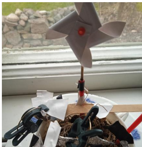
Figure 1. LED and Li-B at left. PPB on heated foundation (heat-element below, cold window at rear) and with foil capacitor not tightly attached. In operation for 24 weeks, since 16/10, (after 26/1, with a clamp, also on the foil)
