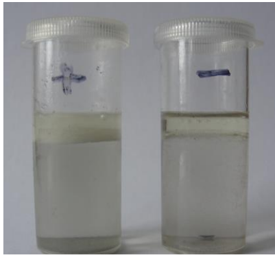
Figure 3. Suspensions formed after intensive mixing of oils with positively charged water do not stratify for hours and, accordingly, retain their milky white or yellowish color (left), unlike suspensions formed after intensive mixing of the same oils with negatively charged water, which stratify within minutes (right) [11, 19].
