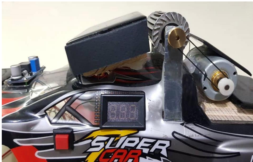
Figure 19. Preventing the damper from hitting the passing air with the turbine
