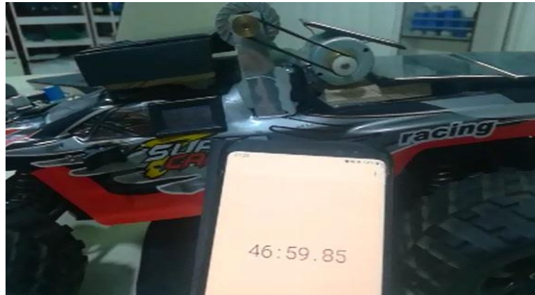
Figure 18. The moment of the end of charging the car battery in the turbine performance test
