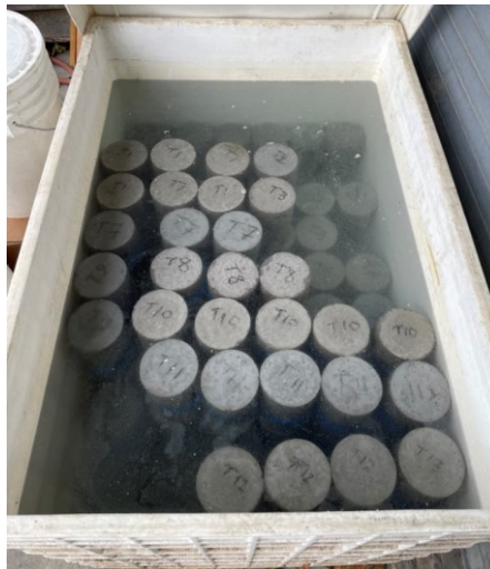
Figure 2. Curing Box for the 12 Mixtures.
