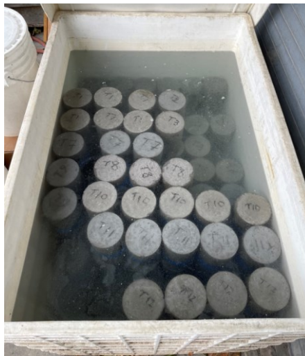
Figure 2. Curing Box for the 12 Mixtures.
